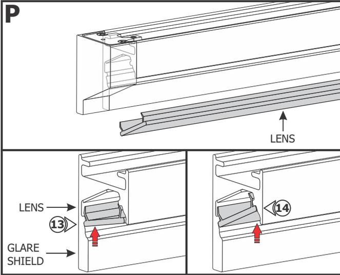
**13:** If the lens is not pre-installed, first push the lens into the glare shield side of the channel.
