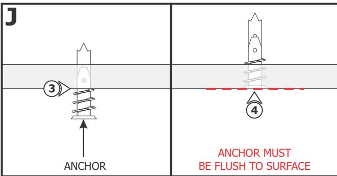
**NOTE:** Steps 3 and 4 are for drywall mounting. Omit these steps if mounting the clips to a wood surface directly.
