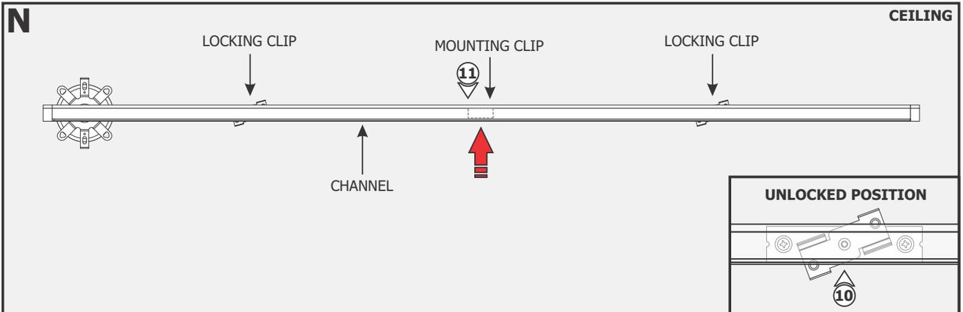
**10:** Make sure the locking clips are in the unlocked position before installing the fixture to the mounting clips.
