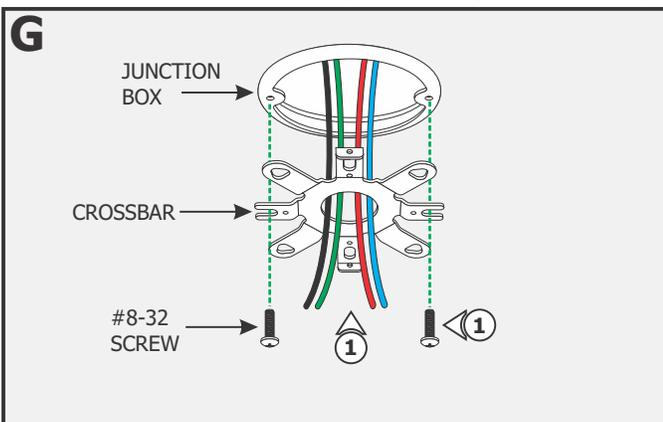
**NOTE:** Remote power supply must be installed within 40ft of junction box. Ensure remote power supply wires are present in the junction box. Refer to instructions provided with the power supply.
