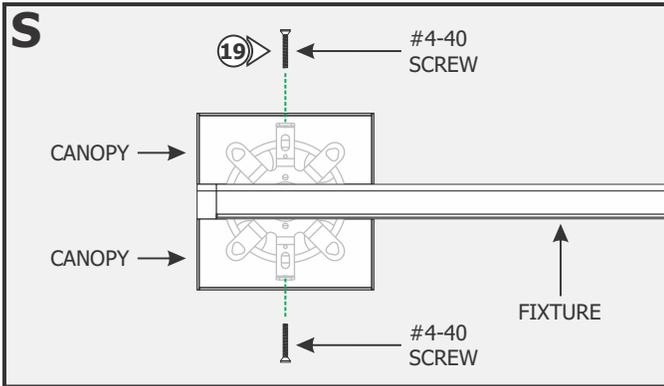
**19:** For 4" Square Split Canopy installations, place each canopy piece against the fixture and align the canopy holes with the crossbar holes. Secure the canopy pieces in place with the two #4-40 screws and 1/16" Allen wrench provided.
