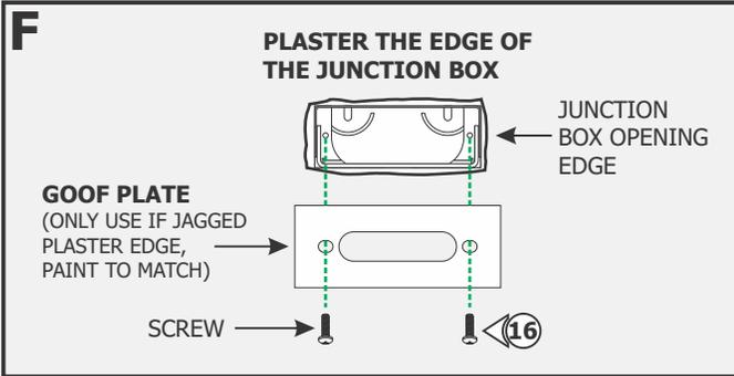
**16: Optional:** Use the Goof Plate if the junction box opening has imperfection/ jagged edges. Install the provided goof plate (paint to match prior) with the two screws.
