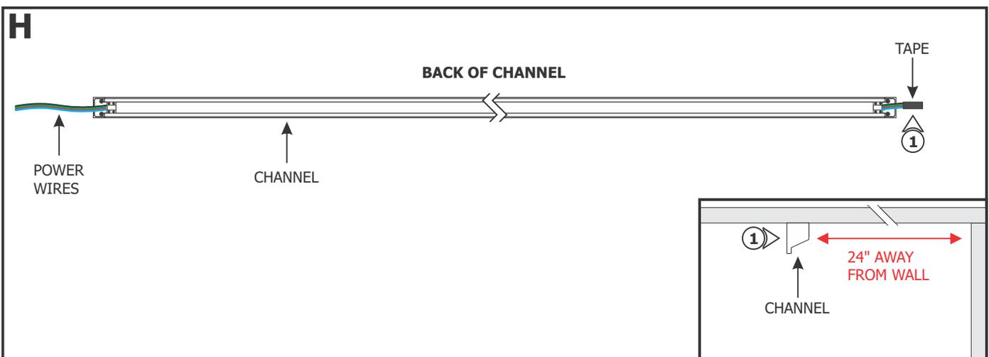
**1:** The Wall Wash channel mounts in one direction, 24" away from the wall to properly light the desired area. Choose the power wires on one end that is closest to the junction box. Cut the unused wires leaving 2" exposed. Wrap the end of the unused wires with electrical tape.
