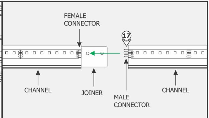
**NOTE:** Omit steps 16 through 18 if the channel is made out of a single piece (120" or less).
