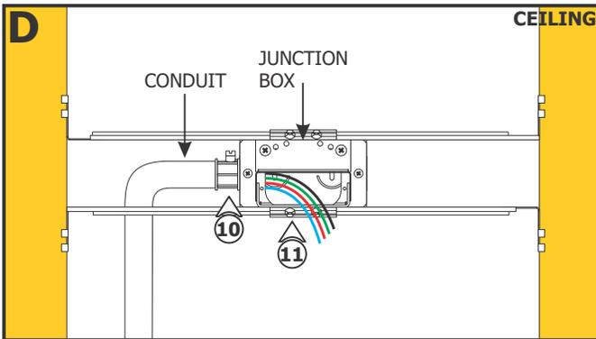
**NOTE:** Remote power supply must be installed within 40ft of junction box. Ensure remote power supply wires are present in the junction box. Refer to instructions provided with the power supply.
