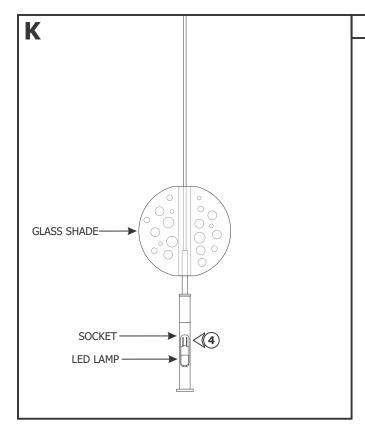
**4:** Push the lamp pins completely into the socket holes.
