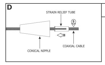
**5:** Feed the coaxial cable through the conical nipple and flared side of the strain relief tube. Slide the conical nipple and strain relief tube down the coaxial cable.
