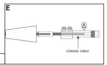
**6:** Feed the coaxial cable into the coaxial fixture connector. The coaxial cable will come to a stop point.
