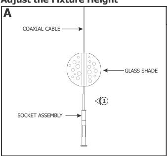
2: Cut the coaxial cable to the desired height (H) with a sharp cutter. The overall fixture height is measured from the bottom of the glass shade to the end of the coaxial cable.
