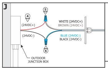
**NOTE:** Outdoor electrical connections must be made inside a waterproof junction box or using waterproof wire nut connections.
