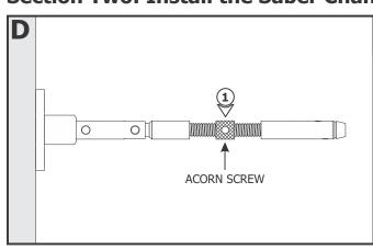
**1:** Unscrew the acorn screw on the turnbuckle body to its full extension for maximum adjustments.
