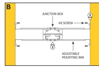
**NOTE:** The adjustable mounting bars mount to joists that are spaced 14.5"-25" apart.
