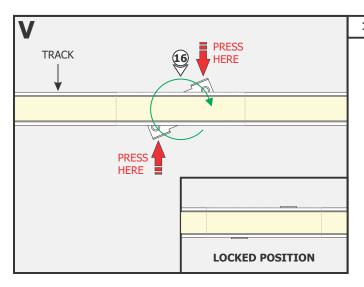
**16:** Twist each locking clip to lock the track in place.
