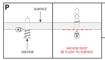
**NOTE:** Steps 4 and 5 are for drywall mounting. Omit these steps if mounting the clips to a wood surface directly.
