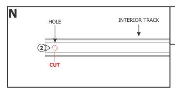
**2:** Drill a hole on the back of the track that will be placed over the junction box to route power to the installation.
