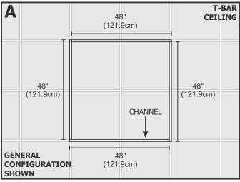
1: Lay out all channels on the floor as a guide to determine where the system will be located on the T-Bar Ceiling.
