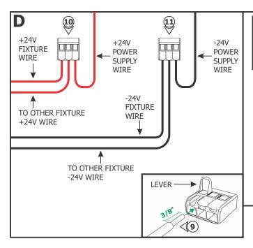
**NOTE:** Depending on the rated wattage of the individual fixtures, the fixtures would share a power supply or be powered individually. When sharing a power supply among fixtures, make sure they are connected in parallel to the output of the power supply.
