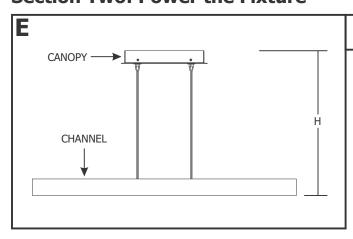
**1:** Determine the fixture height (H), from the bottom of the channel to the top of the canopy.
