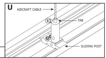
**5:** Insert the aircraft cable through the top of the tab on the sliding post.
