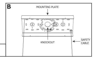
2: Select the appropriate knockout on the mounting plate and remove it using a flathead screwdriver or other appropriate tool.
