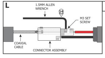
**14:** Use the provided 1.5mm Allen wrench to replace and securely tighten the M3 set screw.
