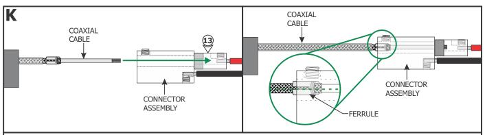
13: Insert the coaxial cable into the coaxial connector until the wires of the center conductor are visible through the M3 set screw hole.
