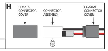
**8:** Unscrew the coaxial connector covers and remove from the connector assembly.
