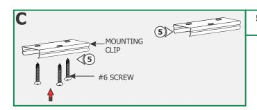
**5:** Line up the mounting clips to the anchors and secure it to the anchors by tightening the three #6 screws to each clip.
