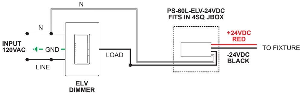
**SAMPLE WIRING DIAGRAM FOR LZUD**
