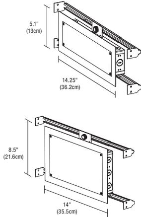
**In-Wall Mounting Kit:** Includes power supply, box cover and stud hangers for installing Junction Box in wall. Select "IW" in the options section of compatible power supply ordering codes if an In-Wall Mounting Kit is needed.
