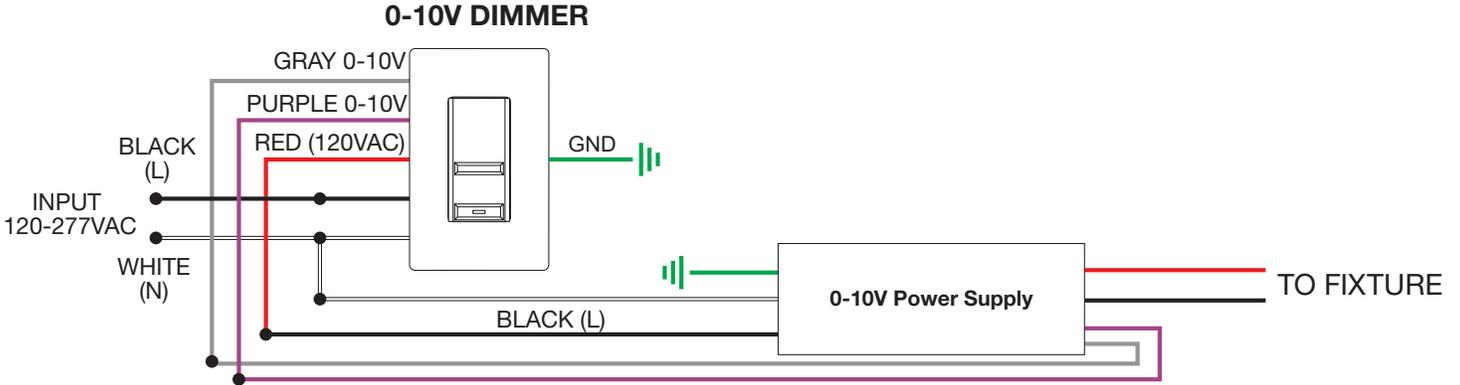
**SAMPLE WIRING DIAGRAM FOR LZUD**
