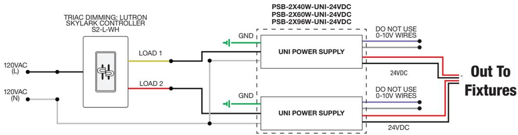
**SAMPLE WIRING DIAGRAM FOR LZ**
