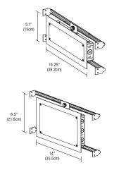
**In-Wall Mounting Kit:** Includes power supply, box cover and stud hangers for installing Junction Box in wall. Select "IW" in the options section of compatible power supply ordering codes if an In-Wall Mounting Kit is needed.
