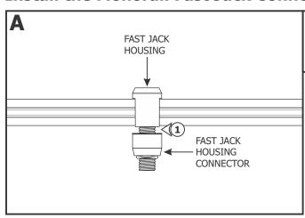
1: Place the Fast Jack housing onto the Monorail and use fingers to tighten the Fast Jack housing connector to the Fast Jack housing. <a href="Make sure that the Fast Jack housing connector">Make sure that the Fast Jack housing connector is not cross threaded.</a>
