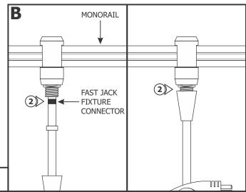
**2:** Use fingers to tighten the Fast Jack fixture connector into the Fast Jack housing connector.
