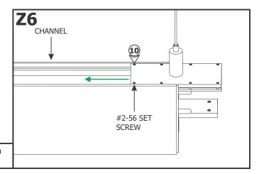
**10:** Loosen the four #2-56 set screws on the top joiner using a 0.035" Allen wrench and slide it inside the channel.
