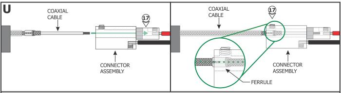
17: Insert the coaxial cable into the coaxial connector until the wires of the center conductor are visible through the M3 set screw hole.
