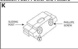
1: Remove the two Phillips screws from the sliding post.
