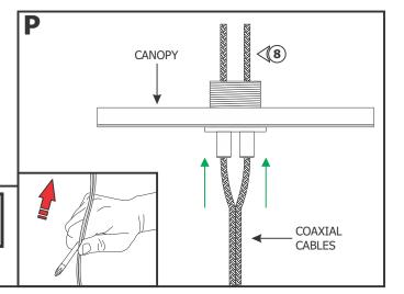
**NOTE:** If cables are curled or kinked, straighten by holding between the shaft of a screwdriver and thumb and pulling the cables through (see inset).
