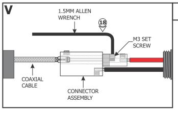
**18:** Use the provided 1.5mm Allen wrench to replace and securely tighten the M3 set screw.
