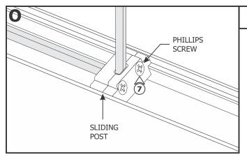
7: Tighten the two Phillips screws on the sliding post to secure it to the channel.
