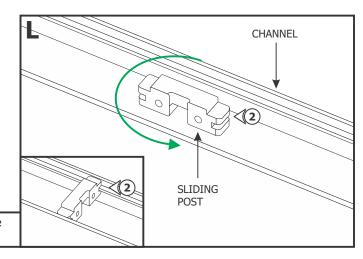
**2:** Place the back part of the sliding post inside the back of the channel and rotate it into place.
