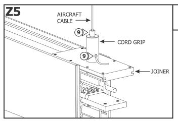
**9:** For each standoff, insert the aircraft cable through the cord grip on the top joiner and pull the aircraft cable out of the side.
