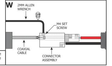
**19:** Use the provided 2mm Allen wrench to securely tighten the M4 set screw until it squeezes the wire ferrule tightly to the coaxial cable.
