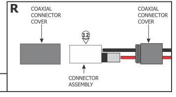
**12:** Unscrew the coaxial connector covers and remove from the connector assembly.
