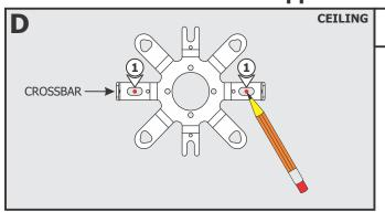
**1:** Mark the points through the crossbar holes onto the ceiling. These points are used for the anchors.
