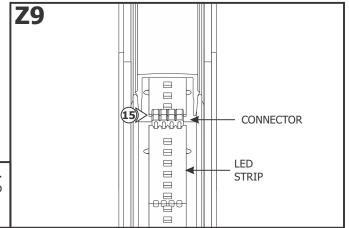
**15:** Connect the male & female connectors of the top LED strips. Firmly press down the adhesive portion of the LED strip onto the channel, making sure there are no air bubbles that can cause surface irregularities.
