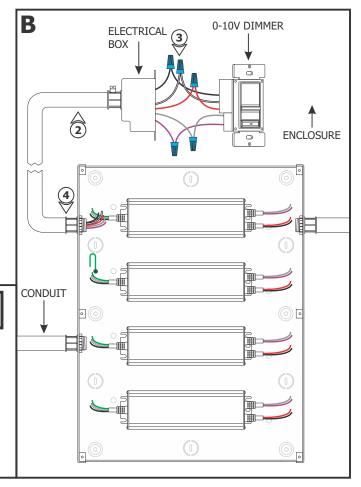
**NOTE:** Refer to wiring diagrams on page 4. Steps 2 through 13 show typical installation for 0-10V dimmers.
