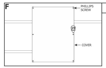
**19:** Replace the power supply cover and secure it by tightening the six Phillips screws.
