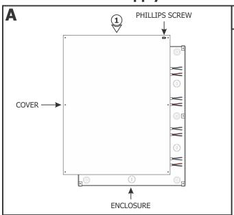
**1:** Remove the six Phillips screws to slide the cover off of the enclosure.
