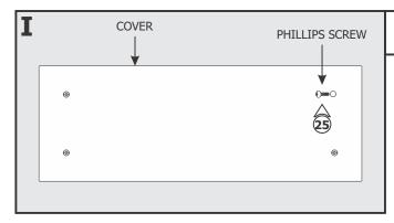
**25:** Replace the power supply cover and secure it by tightening the four Phillips screws.
