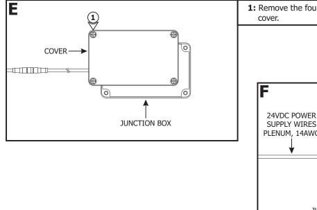
**1:** Remove the four screws on the Junction Box to remove the cover.
