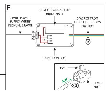
2: Route the 24VDC wires from the fixture to the Junction Box.
