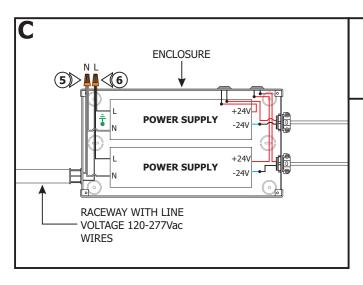
**5:** Connect the white neutral wire from each power supply to the line voltage neutral wire using a wire nut.
