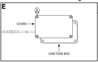
**1:** Remove the four screws on the Junction Box to remove the cover.
