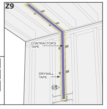
NOTE: Cover the channel opening with blue contractor's tape before plastering.
