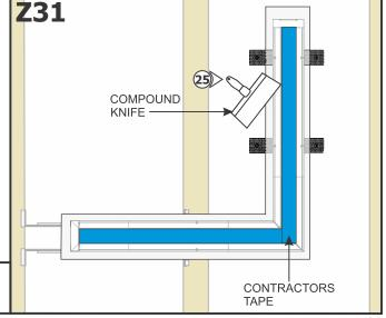
25: Use a compound knife for a smooth compound spread. Sand, paint, and finish the plaster and drywall before removing the blue contractors tape.
