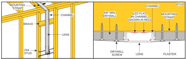
Room-wrapping configurations are used for installations that join runs of **TruLine 1.6** on multiple planes (like a ceiling and a wall) using miter-cut linear sections of channel.
