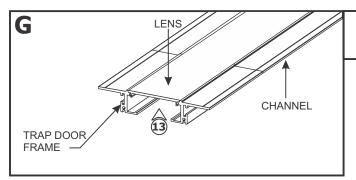
13: Snap the lens into the assembled trap door frame and channel **BEFORE** cutting to length. This ensures a proper fit after installation.
