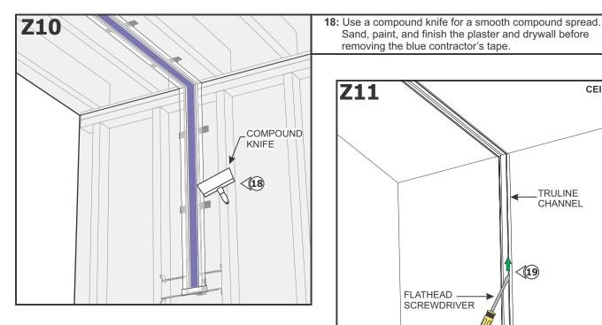
19: Carefully use a flathead screwdriver to remove excess drywall from the internal bevel/edge.
