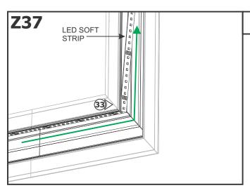
**33:** Continue applying soft strip in side of channel. Carefully bend the soft strip 90° to match the channel corner.
