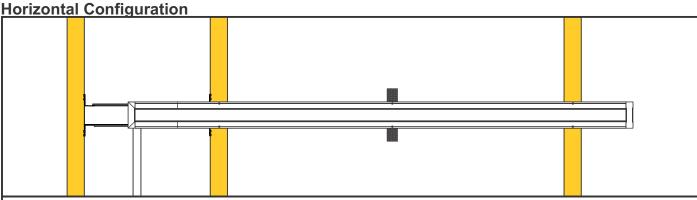
Horizontal installations are linear runs of channel beginning at a junction box and ending at a take-up box on a single surface. Runs can be up to 40' in length and the LED strip lays in the bottom of the channel.
