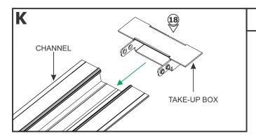
18: Slide the take-up box onto the non-power channel end and tighten the M3 set screws with a 1.5mm Allen wrench.
