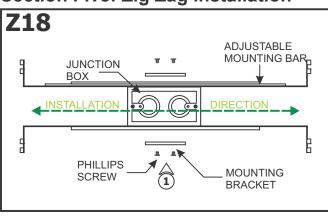
1: Mount each adjustable mounting bar to one side of the junction box and secure them with the mounting brackets and two Phillips screws provided.
