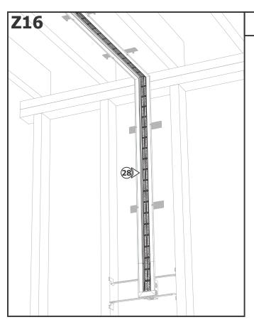
**28:** Repeat Steps 22 through 27 to install the second LED soft strip to the channel.
