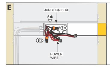
**NOTE:** Remote power supply wires must be present in junction box. Refer to instructions provided with power supply.
