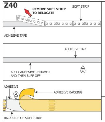
**NOTE:** If relocating the installed soft strip, make sure that the adhesive tape on back of the soft strip covers the entire strip. The adhesive tape isolates the strip from the installation surface. Damaged or inconsistent adhesive tape may cause the contacts on the back of the strip to come in contact with the conductive heat sink which will cause the strip to short and burn. Call Edge Lighting to get replacement adhesive tape and/or optional aluminum heat sink tape (SS-HR-F).
