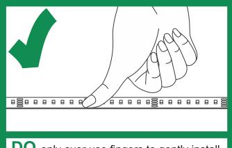
**DO** only ever use fingers to gently install soft strip to a surface **AFTER** cleaning the surface with alcohol.
