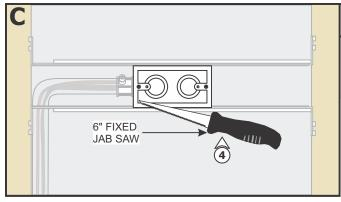
**4:** Cut a section of drywall where the junction box will be located using a 6" fixed jab saw or other appropriate tool.
