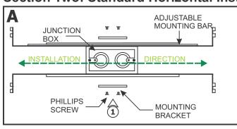
1: Mount each adjustable mounting bar to one side of the junction box and secure them with the mounting brackets and two Phillips screws provided.
