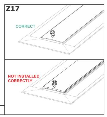
**29:** Snap the lens back onto the channel sections. Ensure lens is fully seated.
