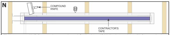
22: Use a compound knife for a smooth compound spread. Sand, paint, and finish the plaster and drywall before removing the blue contractor's tape.
