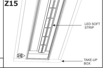
**27:** If required, trim the soft strip on the dashed cutting lines. Place the excess soft strip inside the take-up box.
