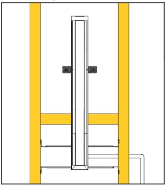
Vertical installations are linear runs of channel beginning at a junction box and ending at a take-up box on a single surface. Runs can be up to 40' in length and the LED strip lays in the bottom of the channel.
