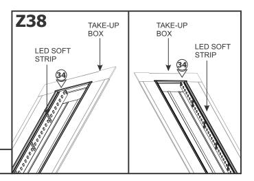
34: Trim excess soft strip along the dotted cutting lines ONLY. Place excess soft strip length into the channel take-up box.
