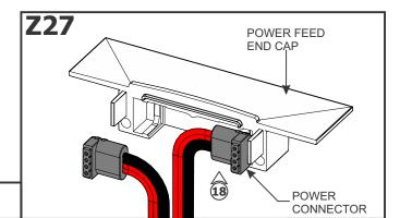
**18:** Place both power connector into the power feed end cap by rotating them 90° to seat.
