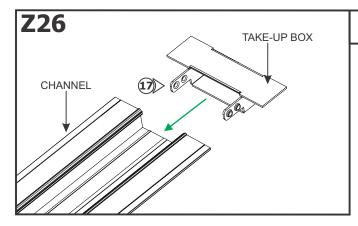
17: Slide the take-up box onto the non-power channel end and tighten the M3 set screws with a 1.5mm Allen wrench.
