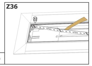
32: Connect and install the second LED soft strip length for the opposite side of the channel by following the same steps as the first.
