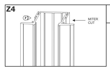
7: Miter cut each section of assembled channel and lens to match the corner angle. In a 90° corner installation as shown, each channel section is cut at a 45° angle to form a complete corner.
