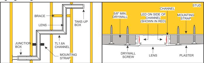
Zig Zag configurations are used for installations that join runs of **TruLine .5A** on a single plane (like a ceiling or a wall) using miter-cut sections of channel.
