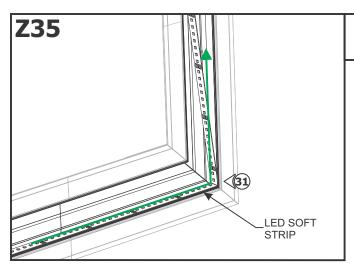
31: Continue applying LED soft strip in the side of channel. Carefully bend the LED soft strip 90° to match the channel corner.
