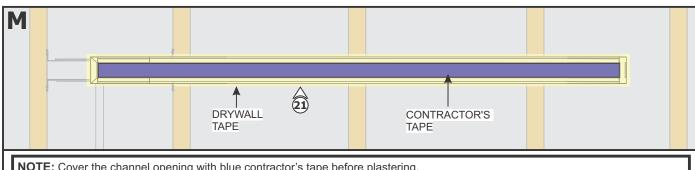
**NOTE:** Cover the channel opening with blue contractor's tape before plastering.
