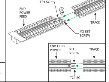
**3:** Align and slide a track over the straight connector (T24-SC) on the End Power Feed. Tighten the set screws using an Allen wrench and the slotted screw on the straight connector using a flat-head screw driver.
