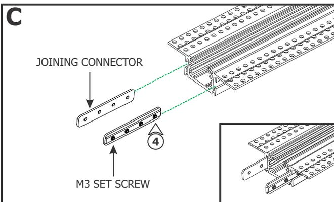
**4:** Insert the joining connectors half way into the L-Connector and tighten the M3 set screws using a 1.5mm Allen wrench.
