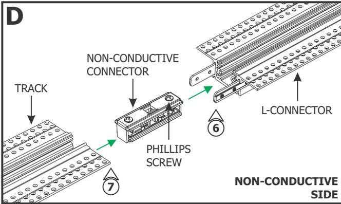
**6:** For the non-conductive side, insert the non-conductive connector half way into one end of the L-Connector. Tighten the screw snugly with a Phillips screw driver (do not overtighten).
