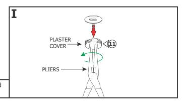
**11:** Use pliers to rotate the plaster cover counter clockwise and remove it. Clean the hole.
