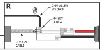
**15:** Use the provided 2mm Allen wrench to securely tighten the M4 set screw until it squeezes the wire ferrule tightly to the coaxial cable.
