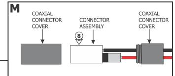
**8:** Unscrew the coaxial connector covers and remove from the connector assembly.
