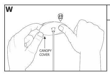
**23:** If necessary, use fingers to push on the perimeter of the canopy cover until it slightly rocks and lift the cover to remove it from the assembly.
