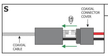
**16:** Replace the coaxial connector cover and tighten into place.
