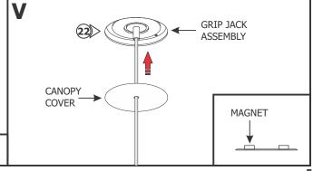
**22:** Place the canopy cover over the grip jack assembly. The magnets on the back will keep the canopy cover in place.
