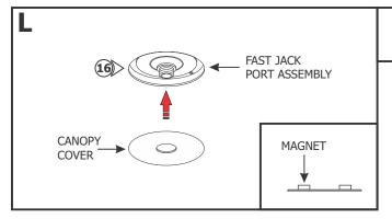
**16:** Place the canopy cover over the Fast Jack Port assembly. The magnets on the back will keep the canopy cover in place.
