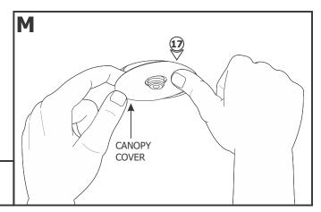
**17:** If necessary, use fingers to push on the perimeter of the canopy cover until it slightly rocks and lift the cover to remove it from the assembly.
