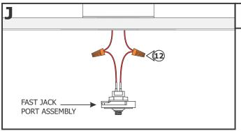
**12:** Connect each transformer wire to one wire of the Fast Jack Port assembly with a wire nut.
