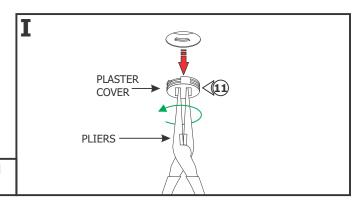
**11:** Use pliers to rotate the plaster cover counter clockwise and remove it. Clean the hole.
