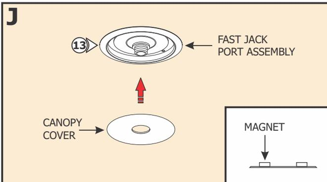
**13:** Place the canopy cover over the Fast Jack Port assembly. The magnets on the back will keep the canopy cover in place.
