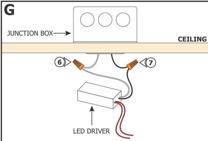
**NOTE:** Steps 6 through 8 are for the 15W or 60W 12V power supply included inside the junction box. Omit these steps if using remote power supply.
