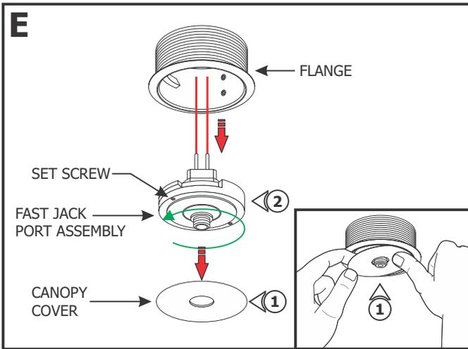
**1:** Use fingers to push on the perimeter of the canopy cover until it slightly rocks and lift the cover to remove it from the assembly.
