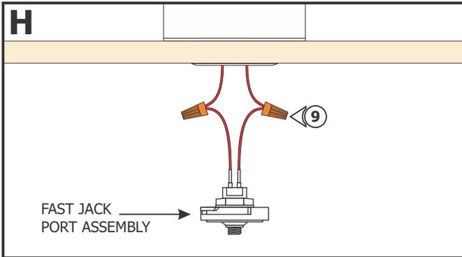
**9:** Connect each transformer wire to one wire of the Fast Jack Port assembly with a wire nut.
