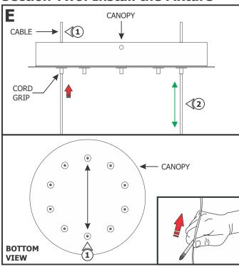
**NOTE:** Cord grips hold the fixture weight only. **DO NOT** pull on the fixture during installation or cleaning which may cause the **power wires to nick and short.**
