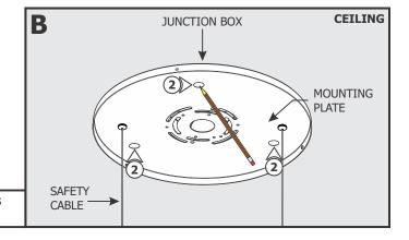
**2:** Align the mounting plate with the junction box. Mark points through the mounting plate holes onto the ceiling.
