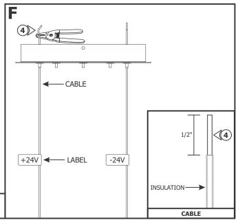
**4:** Use the #16 gauge hole of the AWG wire strippers to strip 1/2" of the outer plastic insulation from the cables.
