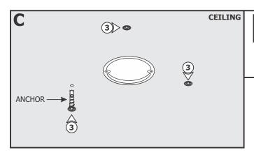
**NOTE:** Step 3 is for drywall mounting. Omit this step if mounting onto a wood surface directly.
