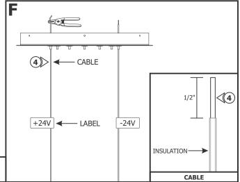
**4:** Use the #16 gauge hole of the AWG wire strippers to strip 1/2" of the outer plastic insulation from the cables.
