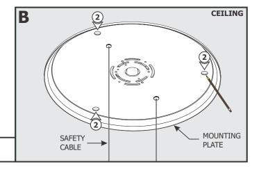
**2:** Align the mounting plate with the junction box. Mark points through the mounting plate holes onto the ceiling.
