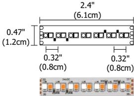
**SS5C Tunable White LED Soft Strip:** Provides variable color temperatures of commercial-grade high CRI LEDs. Flexible copper strip with optically clear protective coating, and industrial strength 3M™ tape backing. Compatible with DMX controls.
