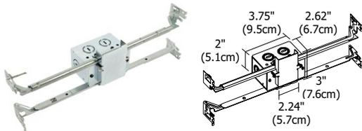
**Junction Box:** Included with End Feed Power Channel Connector. Mounts behind drywall with Adjustable Mounting Bars, and includes a drywall template for accurate installation. Low voltage 24VDC wires from Remote Power Supply connect to LED wires inside box. Junction Box opening is concealed with the Reveal Junction Box cover, and is required at the beginning of each run. Quick
