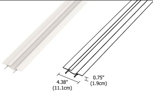
**8 Foot Channel:** 8-foot plaster-in channel. LED Soft Strip (not included) installed flat in the channel. Does not require a lens. Allows for the creation of Reveal BIY systems. May be field-cut to any length, includes Channel Joiners.
