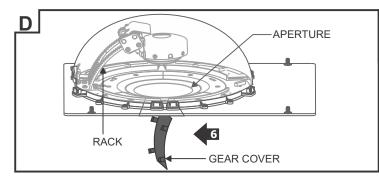
6: Insert the gear cover (make sure the gear cover clips are facing the lamp assembly rack) from the bottom of the aperture.
