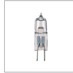
JC20XE/24 20 WATT 200 LUMENS JC10XE/24 10 WATT 95 LUMENS 24V G4 Xenon Lamp JC type G4 Bipin base low voltage 24V Xenon bulb 2000 hours lamp life
