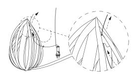
10. Push the steel cable into the nipple at the end of the suspension system.
