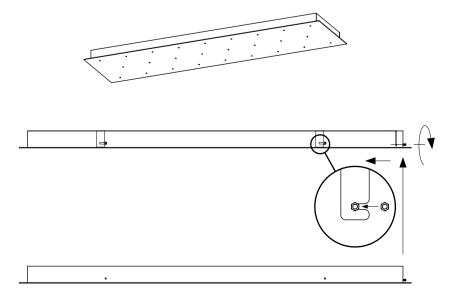
Screw in the locking screw completely.
