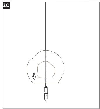
3 Lower the glass shade onto the socket assembly.
