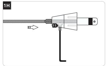
Firmly tighten the set screw on the conical connector.
