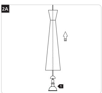
1 Lift the shade up to expose the socket.
