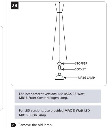
3 Push the new lamp pins completely into the socket.
