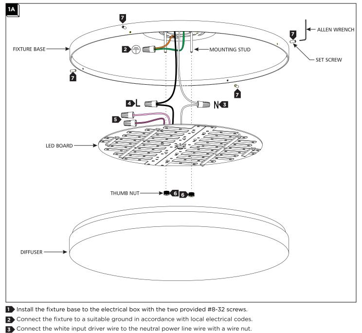
• Connect the black input driver wire to the hot power line wire with a wire nut.
