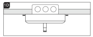
Reattach the transformer to the mounting plate by securing it with the two screws.
