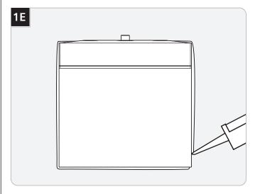
**For wet locations**, caulk around the base with waterproof construction sealant.
