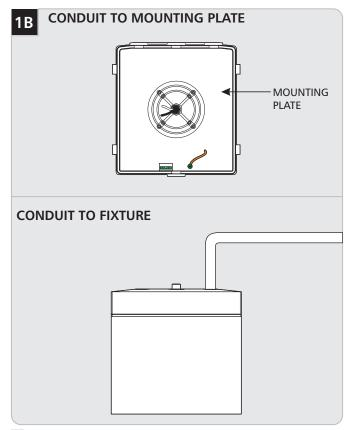
Bring conduit and power lines to the fixture location: conduit may be attached by either the center hole in mounting plate or the any of the plugs on top of the fixture. If using the top plugs, unscrew to remove.
