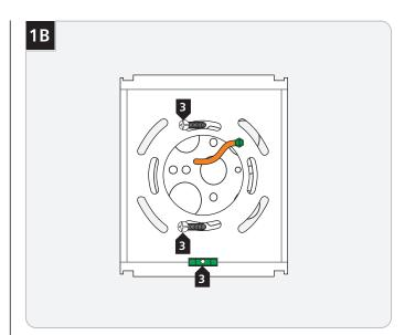
Use the built-in level to ensure the mounting plate is level and secure it to the electrical box using the two provided #8-32 screws.
