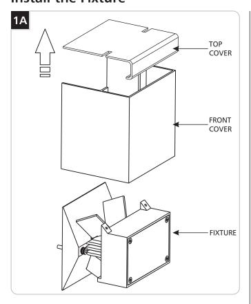
1 If necessary, remove the top cover, then slide the front cover off of the fixture.
