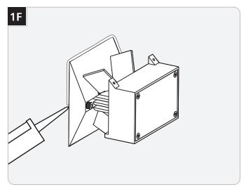
**9** For wet locations, caulk around the base with waterproof construction sealant.
