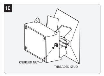
Neatly tuck all wires and wire nut connections into the electrical box, mount the fixture onto the threaded studs, and secure it in place by screwing the knurled nuts onto the studs.
