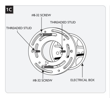
Align the two mounting studs horizontally and mount the mounting plate to the electrical box with the two #8-32 screws provided.
