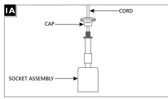
Unscrew and remove the fixture cap from the socket assembly and cord.
