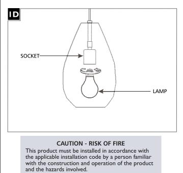
Use minimum 90°c supply conductors.
