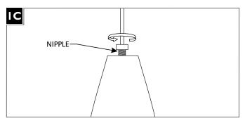
Insert the socket assembly nipple through the top of the shade and secure it in place with the cap.
