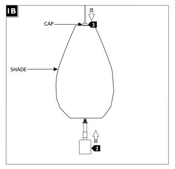
2 Ensure that the washers are in place and feed the fixture cord through the shade.
