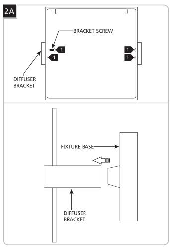
Remove the diffuser bracket from the fixture base by unscrewing the four small bracket screws.
