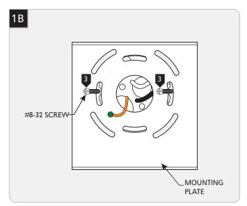
Secure the mounting plate to the electrical box with the provided #8-32 screws.
