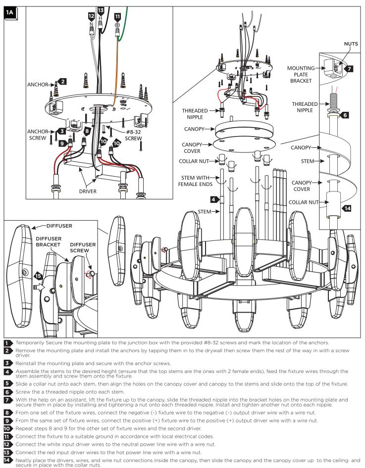
Install a diffuser onto a diffuser bracket and secure it in place with a diffuser screw on each side. Repeat for the rest of the diffusers.
