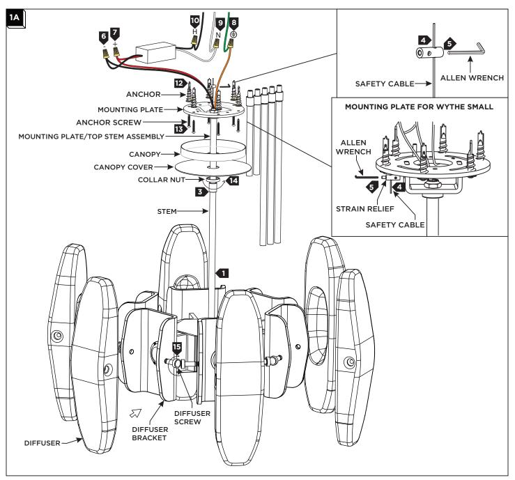
Assemble the stems to the desired height (save the mounting plate/stem assembly for the next step), feed the fixture wires and the safety cable through the stem assembly and screw them onto the fixture.
