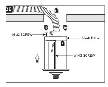
Replace the back ring onto the port so that end of the wing screws are properly placed into the two blind holes.
