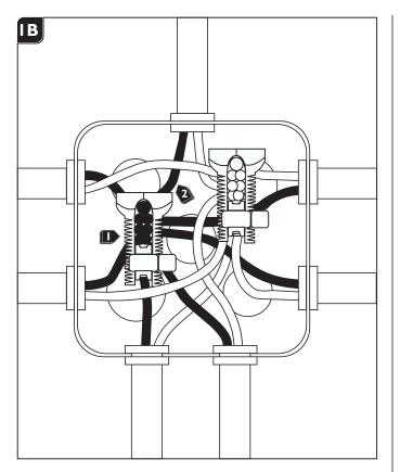
Using a split bolt connector, connect the low voltage hot wire coming from the remote transformer to each hot wire going to the ports.
