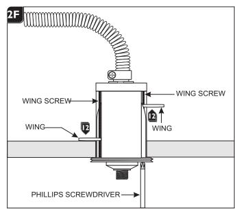
Tighten the two phillips screws with a Phillips screwdriver (an electrical screwdriver will speed up the process) until the wings secure the port into the hole.
