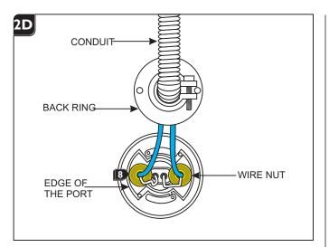
Place the wire nut connections and the port wires properly inside the port. Make sure that the port and low voltage wires are cleared from the edge of the port.
