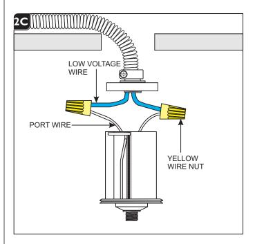
**6** Cut the port wires so that 1-1/2" of it is exposed.
