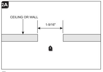
Use a 1-9/16" hole saw to cut out the ceiling or wall where the ports are going to be installed.
