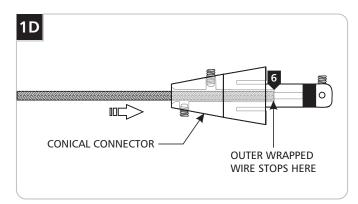
Feed and push the coaxial cable into the conical connector. The coaxial cable will come to a stop point after being inserted 3/4" into the conical connector.
