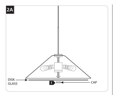
1 Loosen the cap and carefully remove the disk glass to expose the sockets.
