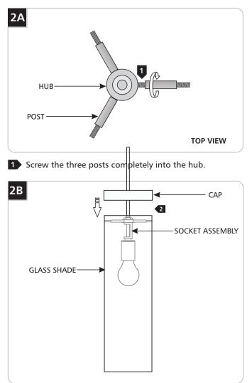
2 Place the socket assembly into the glass shade then place the cap on top of the glass shade.
