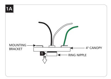
1 Unscrew the ring nipple and detach the 4" canopy from the mounting bracket.
