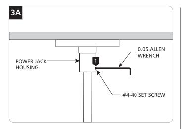
To lock the fixture head in a permanent horizontal position, tighten the #4-40 set screw on the fixture Power Jack housing with the provided 0.05 Allen wrench.
