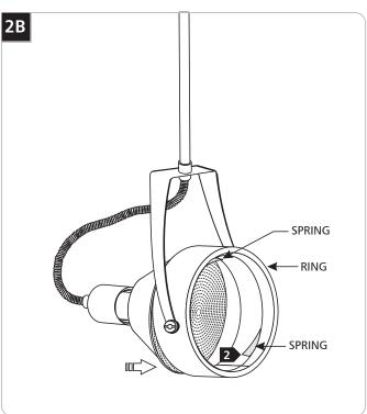
2 Push the lamp edge against the springs inside the ring until the edge of the lamp locks behind the springs.
