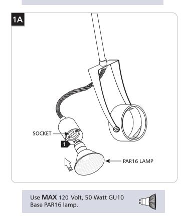
Push the lamp pins into the large portion of the socket slots and rotate clockwise to lock the lamp in place securely.
