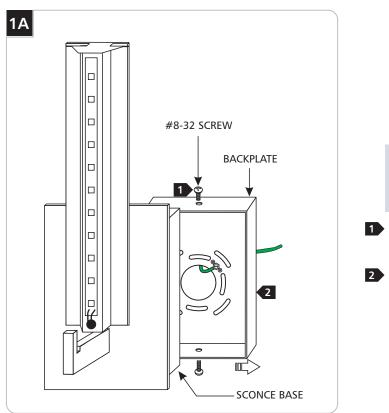
**CAUTION:** When handling the fixture, do not apply pressure to the LEDs. Hold the fixture by the sconce base or aluminum extrusion only.
