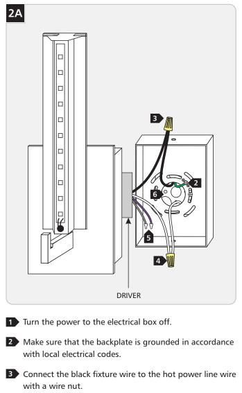
4 Connect the white fixture wire to the neutral power line wire with a wire nut.
