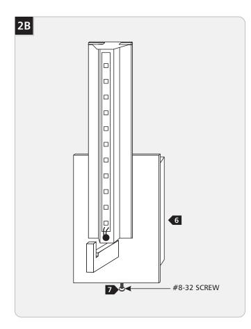
6 Place the sconce base onto the backplate and align the holes.
