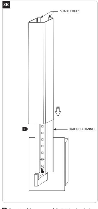
2 From top of the sconce carefully slide the glass shade edges into the bracket channels.
