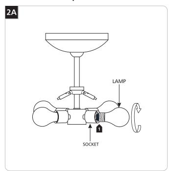
**CAUTION:** To reduce the risk of a burn or electric shock during relamping, disconnect the power to the fixture.
