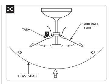
**NOTE:** Assistance will be needed to install the glass shade and to support it while adjusting the aircraft cables to position it in place.
