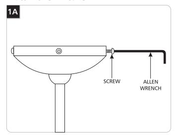
1 Separate the mounting plate from the canopy by removing all four screws with the provided Allen wrench.
