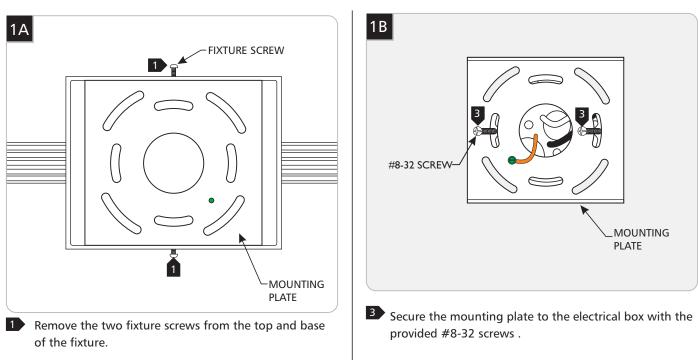
2 Remove the mounting plate from the back of the fixture.
