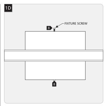
8 Mount the fixture by sliding it back onto the mounting plate and reinstalling the two fixture screws (reversal of figure 1A).
