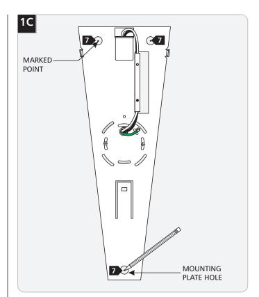
Mark three points onto the wall through the mounting plate holes.
