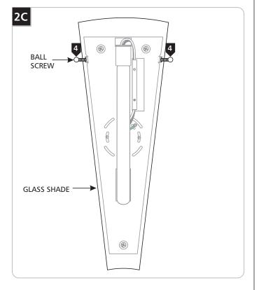
4 Slightly screw (Do Not Tighten) the ball screws through the glass shade holes into the cage nut holes so that the glass shade is held in place.
