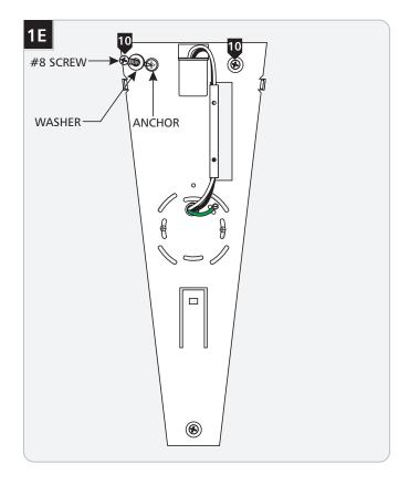
**10** Secure the mounting plate to the anchors with the #8 screws and washers.
