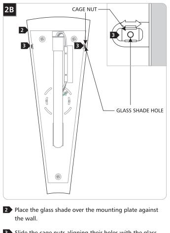
3 Slide the cage nuts aligning their holes with the glass shade holes.
