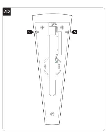
5 Firmly push the glass against the wall and finish tightening the ball screws.
