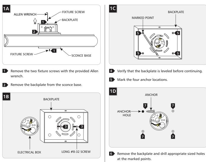
Temporarily mount the backplate to the electrical box with two long #8-32 screws.
