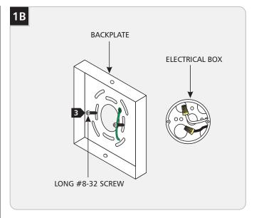
Mount the backplate to the electrical box with two long #8-32 screws.
