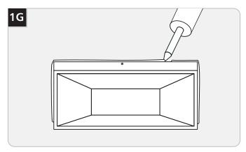
**14** For wet location installation, caulk around the mounting base with waterproof construction sealant.
