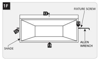
Re-install the shade to the fixture base and secure it with the four fixture screws using the provided Allen wrench.
