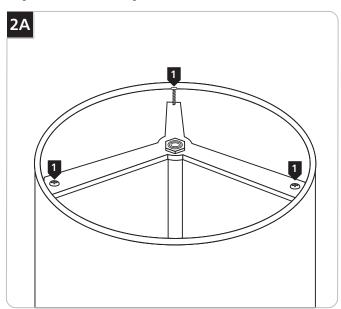
1 Carefully remove the shade by unscrewing the three mounting screws on top of the fixture.
