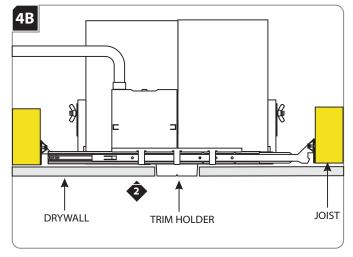
Align the cut out section of drywall with the trim holder and install drywall.
